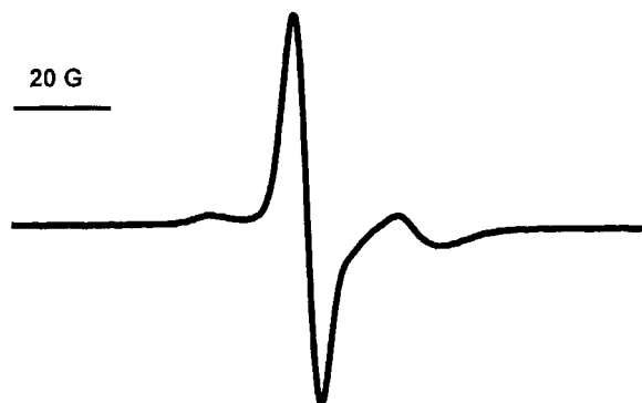
Figure 9 ESR spectrum for the CGCTiMe 2 /B(C 6 F 5 ) 3 system in toluene recorded at [Ti] 0 = 2 × 10 -2 M, B/Ti = 1.0 (molar), t = 20 min, and T = 100°C.
